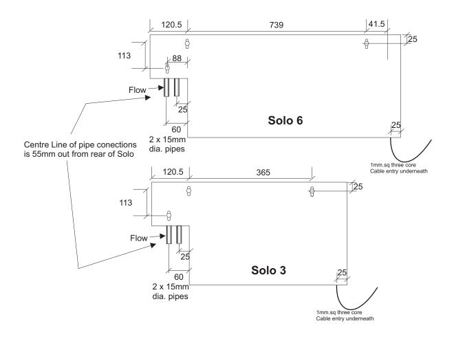
Pipe connections are as shown, and are either 15mm dia. Plastic or copper. Please note flow connection on LHS.
